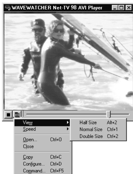
Figure 3-11 Drop-down control and configuration options optimize playback quality.
